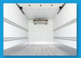
Thermal-efficient composite panels on the roof, walls and floor that maintain the inside temperature from 0 °F to 32 °F far more efficiently than conventional panels.
