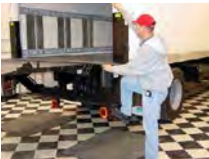
Step #4: Unfold any gate extensions
