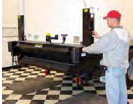
Step #2: Release gate from stored position
