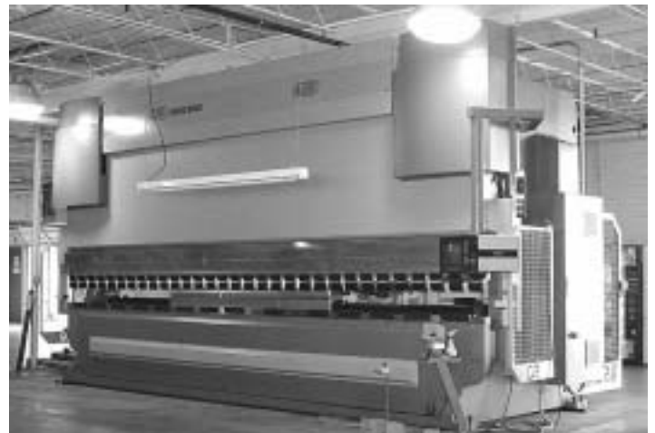
Brake press weighs about 56 tons, has a bending force up to 440 tons and can bend parts that are up to 20 feet, four inches long.
