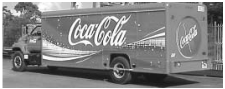
A 10.5-bay all-aluminum Coca-Cola body in Venezuela. Panamco has continued to upgrade its fleet with similar units after its acquisition by FEMSA.
