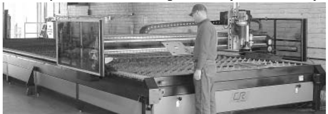
New plasma cutter facilitates a 10- by 40-foot sheet, versus 8 by 16 feet on the previous machine.
